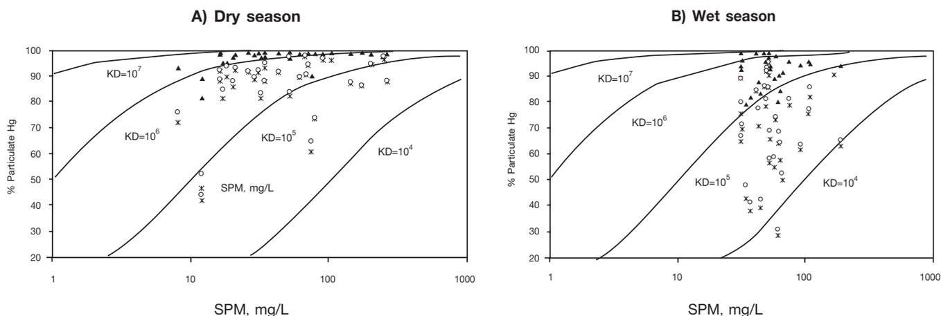
**Figure 8** The variation in percentage of particulate Hg with suspended particulate matter (SPM)
