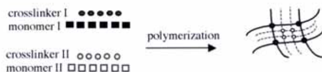
Figure 1 A schematic of two basic polymerization methods of IPNs : (a) Sequential IPN, (b) Simultaneous interpenetrating polymer network (SIN) (Sperling, 1981).
