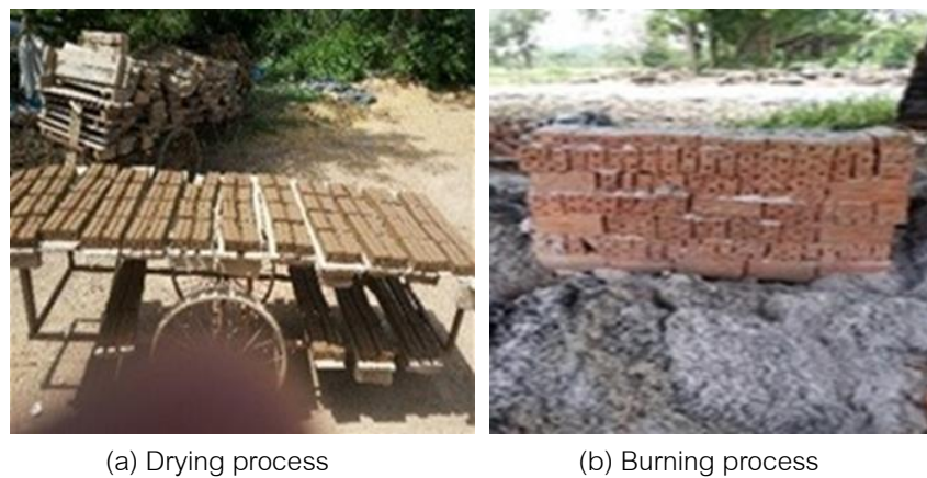
Figure 3 Drying and burning process
