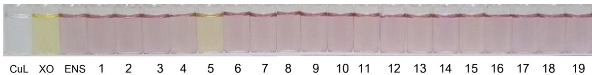
Figure 5 Colour change of [CuL:XO] ensemble solution in the presence of various anions and OPP in 80:20% (v/v) DMSO:H 2 O 10 mM HEPES buffer pH 6.4. 1) atrazine 2) dichlovos 3) ethion 4) glufosinate 5) glyphosate 6) malathion 7) parathion 8) phosphate 9) pyrophosphate 10) triphosphate 11) adenosine monophosphate 12) adenosine diphosphate 13) adenosine triphosphate 14) acetate 15) glycine) 16) malonate 17) oxalate 18) citrate 19) chloride.
