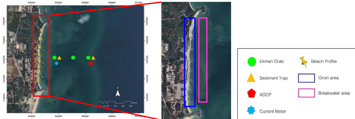
Figure 3 current velocity & direction, sediment sampling and coastal morphological measurement station (Source : modify from Google Earth)
