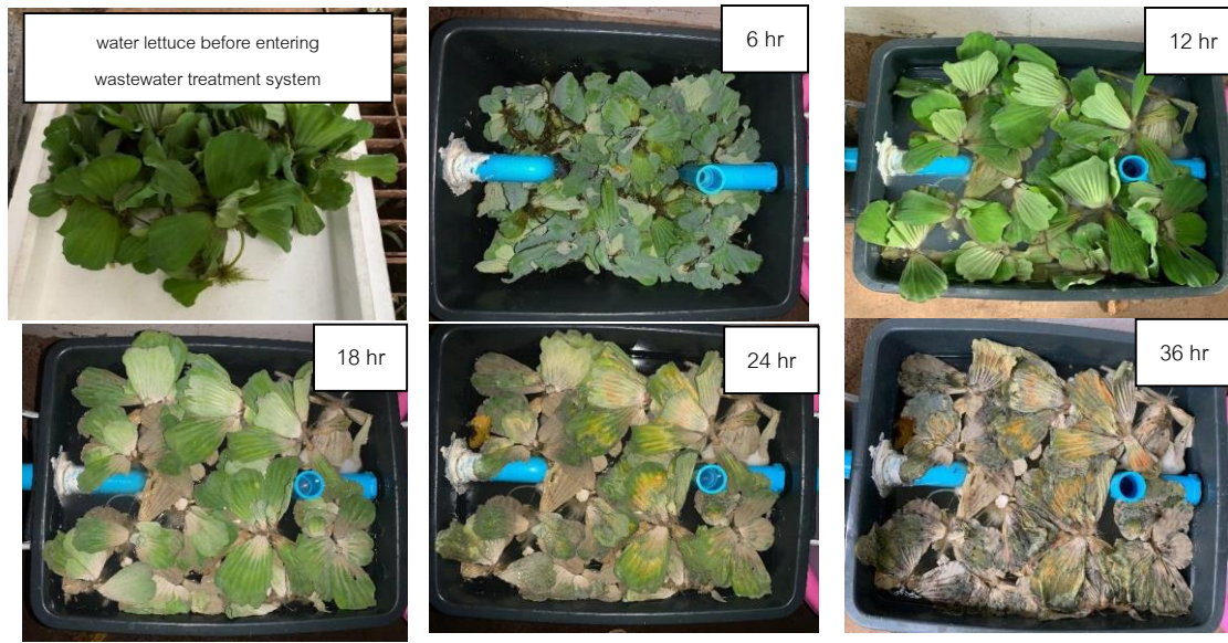
Figure 7 Water lettuce after treated wastewater from Fermented Rice Noodles Factory at different hydraulic retention times
