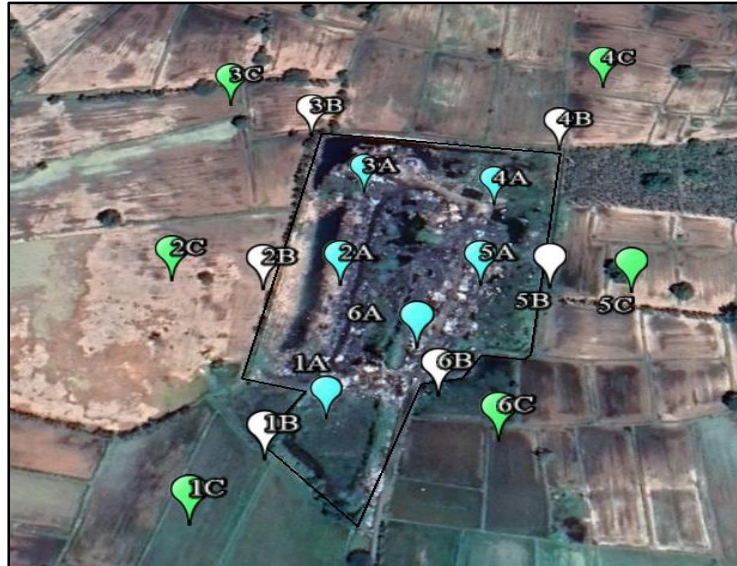
Figure 1 Soil Samples Collection Spots within Waste Disposal Site and the Surrounding Rice Paddy Fields
